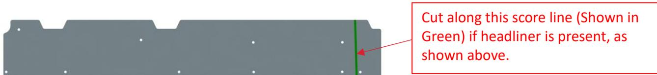
**Step 4:** Bring the (P1A) Liner into the vehicle and align the holes on the panel with the ones present on the vehicle's body.
